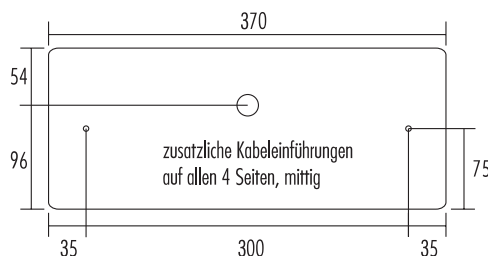
Bohrabstände PF Wand/Decke / drilling holes PF wall/ceiling
